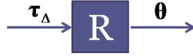
Figure 3. Block diagram of linear MIMO structures using vector and matrix notation: \mathbf{R}(s) is the transfer function matrix from the commanded torque perturbations, \boldsymbol{\tau}_\Delta , to the angular displacement, \boldsymbol{\theta} .
